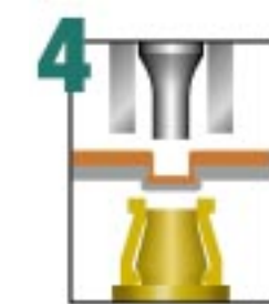
The tooling unclamps the material and the part is easily removed.
